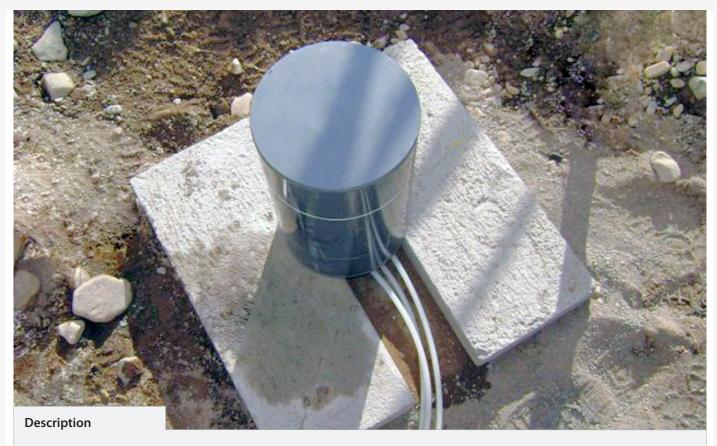
The Hydraulic Overflow Settlement Cell is used for measuring vertical movements and controlling subsidence.
